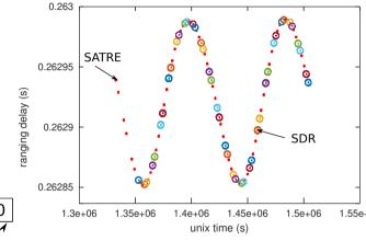
**Result**: time of flight (ranging) measurement consistent with proprietary SATRE modem communication, but the **satellite is moving by**  $\pm 75 \mu s$  (150  $\mu s$ =45 km)!
